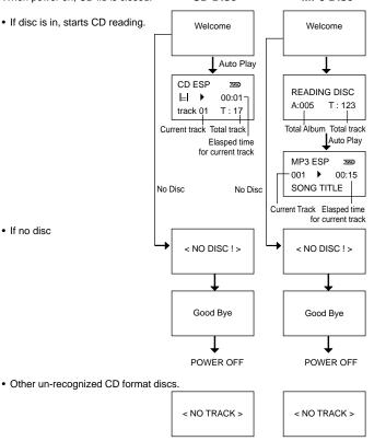
NOTE: On rare occasions, the unit may display <Can Not Read> or <READING DISC> or other messages. This condition is caused by a CD with an unrecognized format. If the player is unresponsive or appears to be locked up, simply open the CD door, remove the CD and replace with a CD containing a supported format.
